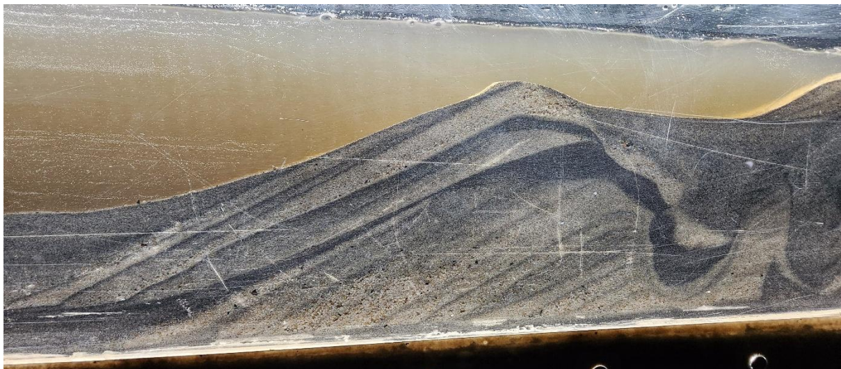
Sands self-sort into layers in a matter of minutes in the strata machine
